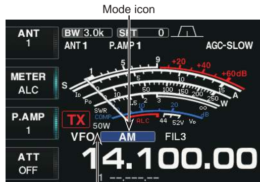
TX power readout
