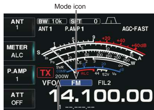
TX power readout
