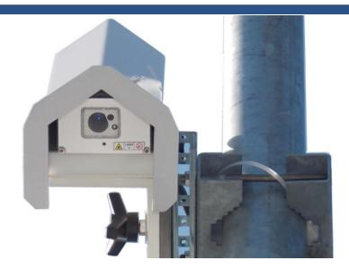
The laser-based snow depth sensor Lufft SHM31 stands for millimeteraccurate snow level detection over long distances in all weather conditions without any maintenance, due to opto-electronic/laser based rangefinder technology.
