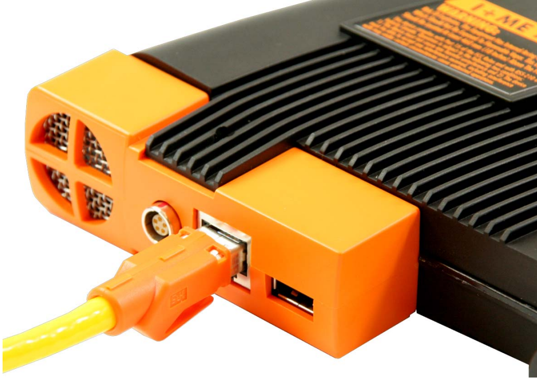
Fig. 5 Ethernet connection ICOM A
