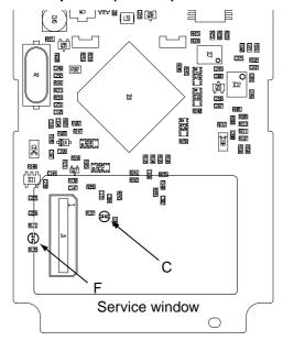
• Cut the junction patterns C and F on the PC board.
