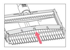
1. Lift the clamping bar at its center and remove it
