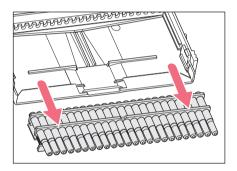
2. Slide the cylinder block straight down and out of the housing case. The lower part can be cleaned.
