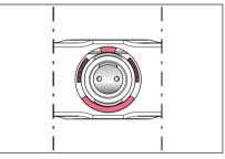
3. View the detached lower part from above. For this, slide the housing case down. Note the exact position of the red marked parts. **The red marked stops on the housing case and the red marked teeth on the inner part are adjacent.** If the stops and teeth are on top of each other after assembly, the housing case has been attached incorrectly.
