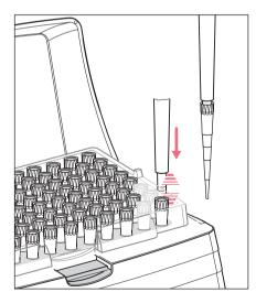
Insert the tip cone of the pipette into the pipette tip using light force to ensure that a sufficiently firm connection is created between the pipette and the pipette tip.
