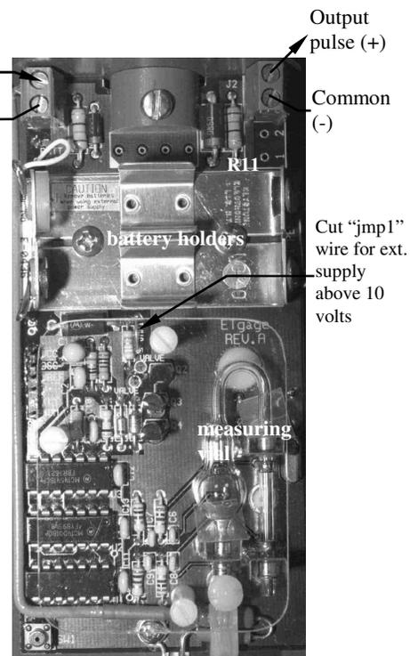
**Signal:** After each 0.01-inch of evaporation, the ETgage's circuit pulls the signal line low for  $2.3 \pm 0.7$  seconds. Normally this line appears as an open-circuit, with infinite impedance. During an output pulse it falls to 35 ohms<sup>1</sup>. The receiving equipment must supply voltage through a pull-up resistor, or other means. Maximum voltage supplied to the signal line should not exceed 30 VDC since larger values will cause an over-voltage current to flow.
