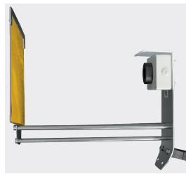
Thank you for choosing Pessl Instruments GmbH iMETOS iSCOUT® Color Trap for Remote Trap Image Monitoring. iMETOS iSCOUT® Color Trap periodically takes high resolution photos of the insect trap. Photos are automatically uploaded to the FieldClimate platform without the need of any user intervention, thus allowing a continuous insect control in the agricultural sector. Device comes with a high-resolution camera and a holder for a sticky plate.
