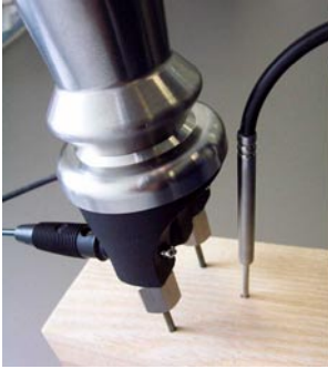
Reciprocating piston electrode GHE91 with temperature-probe GTF38
