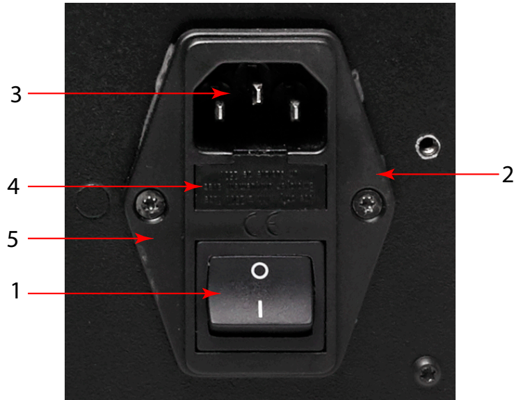
Figure 30 Power Supply Fuse Replacement
