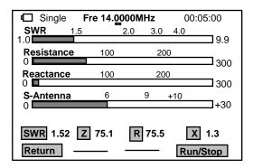
With the generator running, you may change frequency on the fly using the Encoder while watching the display for key points of interest such as resonance (X = 0), minimum SWR, and the antenna's 2:1 bandwidth limits. You may also use the analog bars to provide continuous feedback when adjusting tunable
