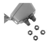
Run the sensor cables through the gland caps and then through the gland.
