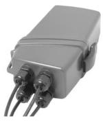
**IMPORTANT!** The enclosure can only be waterproof if all the connections are snug. If you can easily slide a cable in or out, water will be able to enter the enclosure. Tighten the gland cap. Make sure that any unused glands are secured with gland plugs.
