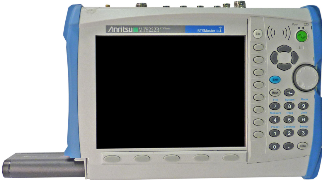
Figure 4-4. Removing the Battery
