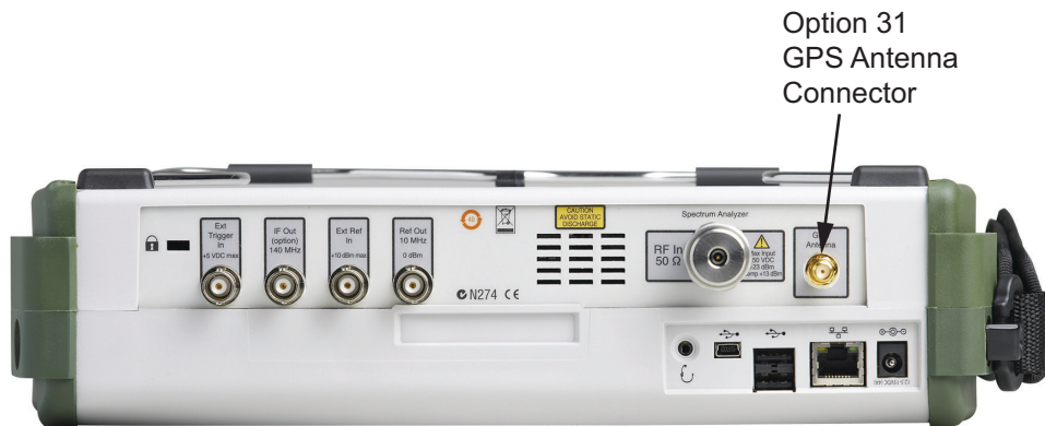
Figure 5-1. Remove Option 31 Lock Nut and Washer
