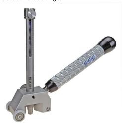
The well proven ERICHSEN Hardness Test Pencil 318 has been improved decisively years ago in the form of a parallel design, Mod. 318 S, with rolling test head.
