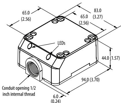
Suggested mounting: M5 or SAE#10 cap screw should be used with a split lock washer to install the unit.
