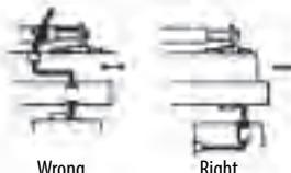
The location of oiltight limit switches and the method of connecting them should be such that condensation in the conduit cannot enter the switch enclosure.
