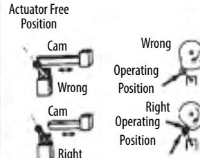
A limit switch actuator must be allowed to move far enough for positive operation of the contacts.
