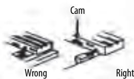
Limit switches should be mounted rigidly and in readily accessible locations with suitable clearances to permit easy service and replacement when necessary. Cover plates should face the maintenance access point.
