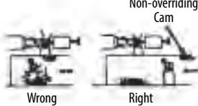
Limit switches should be placed in locations where machining chips do not accumulate under normal operating conditions
