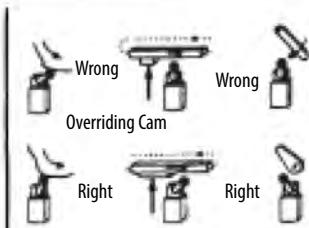
Cam or dog arrangements should be such that the actuator is not suddenly released to snap back freely.
