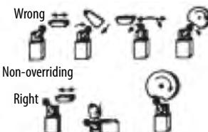
For limit switches with lever actuators, the actuating force should be applied as nearly perpendicular to the lever as practical and perpendicular to the shaft axis about which the lever rotates.
