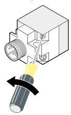
Pull head and mounting base gently apart and twist to new position. Note: do not pull on connecting cable. Damage to unit may result.
