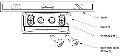
Figure 1. Mounting the bracket Copyright © 2008 - 2009 Airmar Technology Corp.
