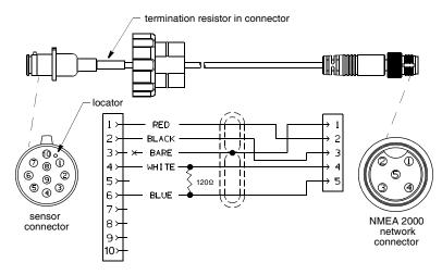
Figure 7. NMEA 2000 Sensor Cable [10m (33') shown] Copyright © 2009 - 2011 Airmar Technology Corp.
