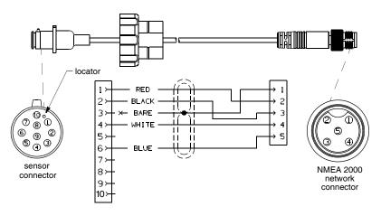
Figure 6. NMEA 2000 Sensor Cable [6m (20') shown] Copyright © 2008 - 2011 Airmar Technology Corp.
