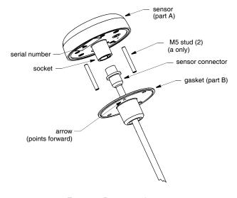
Figure 2. Preparing the sensor Copyright © 2008 Airmar Technology Corp.
