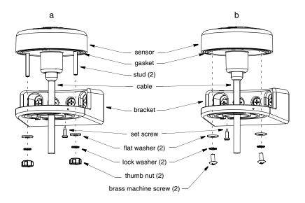
Figure 3. Installing the sensor in the mounting bracket Copyright © 2008 - 2009 Airmar Technology Corp.
