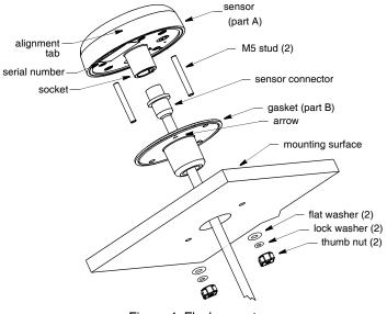
Figure 4. Flush mount Copyright © 2008 Airmar Technology Corp.
