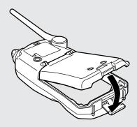
The life of alkaline batteries is approximately 60 hours and the life of an optional UPB-1 battery pack is approximately 24 hours; where the ratio of transmission, reception, and standby periods is 1:1:8.
