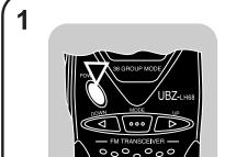
Press the **POWER** switch for more than 1 second to turn the transceiver power ON.
