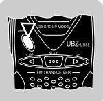
To turn the transceiver power OFF, press the **POWER** switch for more than 1 second.
