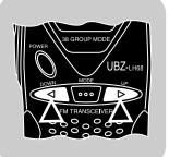
Press the **UP** or **DOWN** key to select the operating channel (1 to 68).
