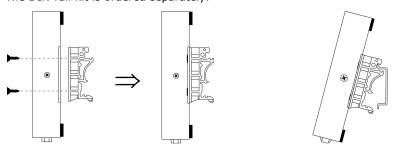
**Mounting on the wall:** You will first need to attach the mounting plates to the unit. Place four screws in the wall and slide the unit onto the screws as shown.
