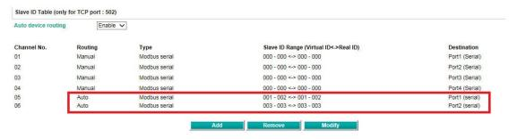
This snapshot shows the routing mechanism is in Auto mode, and the gateway detects that slave ID 1 and 2 are connected in port 1 and slave ID 3 is connected in port 2.
