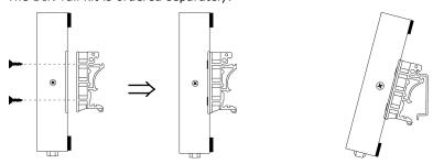
**Mounting on the wall:** Place two screws in the wall and slide the unit onto the screws as shown. The head of the screws should be 5 to 7 mm in diameter, the shaft should be 3 to 4 mm in diameter, and the length of the screws should be at least 10.5 mm. Make sure to leave about 2 mm of space between the head and the wall.
