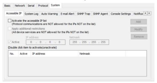
The Accessible IP List function allows you to add or block remote host IP addresses to prevent unauthorized access. Access to the MGate MB3000 is controlled by IP address. That is, if a host's IP address is in the accessible IP table, then the host will be allowed to access the MGate MB3000. The different restrictions are listed in the table below (the checkbox **Apply additional restrictions** can only be activated if **Activate the accessible IP list** is activated.
