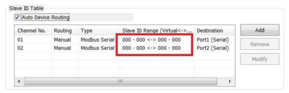
Users can only check the result of auto-detect routing table through the web console.
