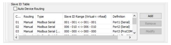
Select the second channel and click **Modify**. Since the virtual ID recognized by the Modbus master is 2, and the real slave ID of the device B is ID 1, the offset should be set as -1.
