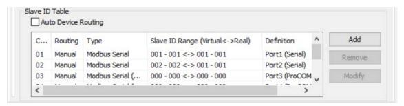
Now, the Modbus master can send a request with slave ID 1 to Modbus device A connected to serial port 1 as well as send a request with slave ID 2 to the Modbus device B connected in serial port 2.
