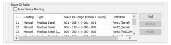
Select the first channel and click **Modify**. The Slave ID represents the Virtual ID recognized by the Modbus master.
