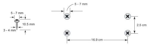
The head of the screws should be 5 to 7 mm in diameter, the shaft should be 3 to 4 mm in diameter, and the length of the screws should be at least 10.5 mm. Make sure to leave about 5 mm of space between the head and the wall.
