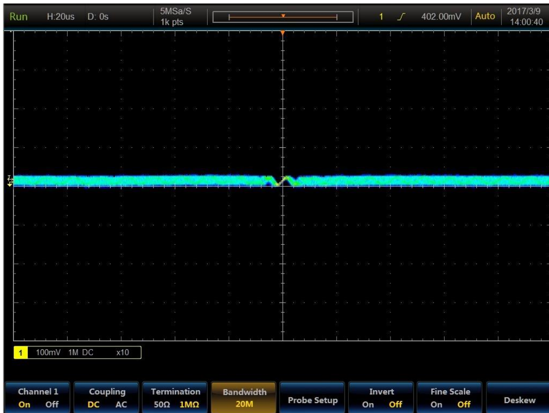
Trigger sensitivity can be adjusted continuously, the highest reaches 0.1 div.
