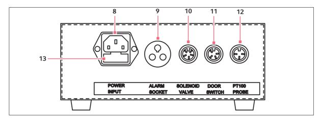
Fig. 3-2: Back view of the LN<sub>2</sub> Back-up System
