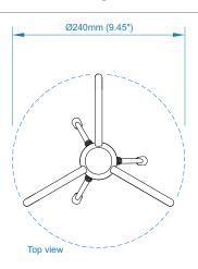
Positions for three off bolt fixings with  $\emptyset$ 7.0mm (0.27") max. thread. on a p.c.d. of 85mm (3.35")
