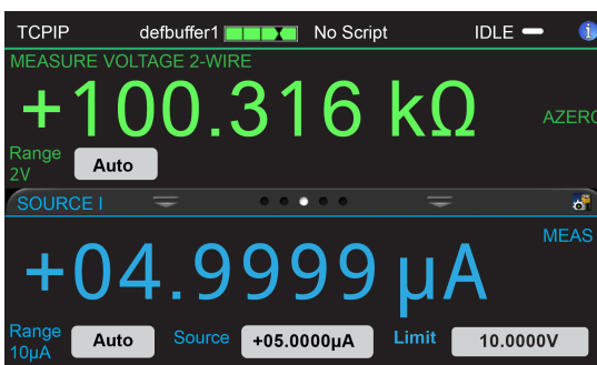
Figure 68: Resistance measurement SIMV and read ohms
