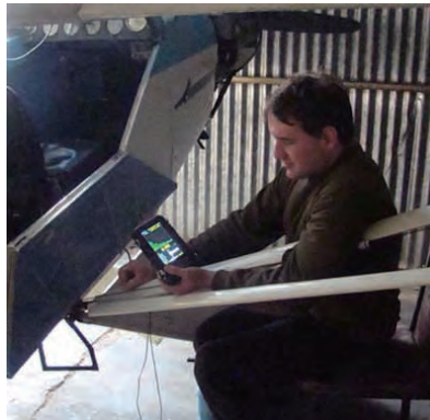
CTS-59 measures the wing struts from a Piper PA-11 small aircraft
