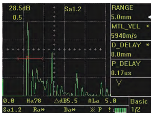
(Bottom echo of a 1.2mm steel plate)
