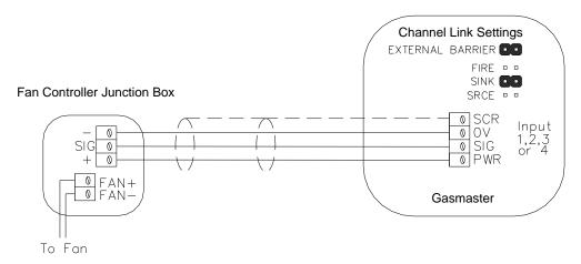
Connect the ESU fan controller to the **Vortex** control panel as shown. Refer to the Appendix C of this manual for details on how to configure the input channel.
