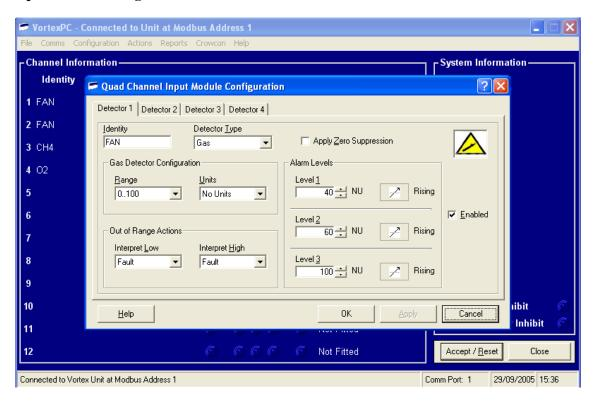
**2. Fault ('Fan Stopped or Disconnected') relay configuration**: the selected Fault relay <u>must</u> be set with a 3 second off delay. Level 1 and Level 2 'Fan Slow' and 'Fan Stalling' alarms can be set as latching or non-latching as required.
