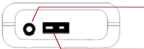
**Output:** Connection for optically isolated interface adapter or for analog output (please refer to chapter 8)
