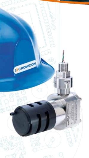
IREX is an innovative infrared (IR) flammable gas detector designed specifically to directly replace pellistor (catalytic bead) type flammable gas detectors. IREX operates from control systems designed solely for use with pellistor-based gas detectors: it produces a mV Wheatsone Bridge type signal (as per a pellistor) and operates from as little as 2.9Vdc. IREX is supplied with an M20 type fixing enabling originally installed detector junction boxes and cables to be retained.
