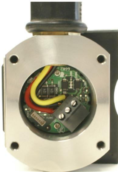
*Diagram 4: IREX rear view with back-plate removed*
