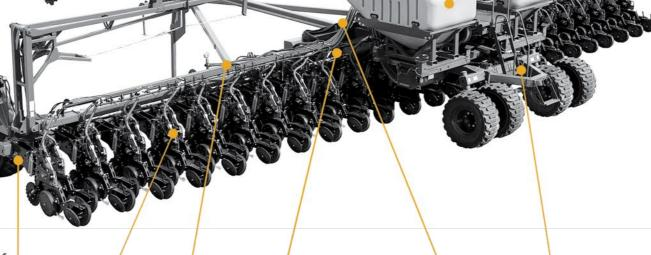
The IntelliAg Air Cart Control (ACC) System allows for full utilization of a 1 to 4 bin air cart. The system monitors seed or fertilizer traveling through the air system to ensure the material is getting to the soil and is not being trapped in a hose.
