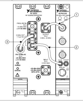
Figure 4. NI 5661 Front Panel Interconnection
