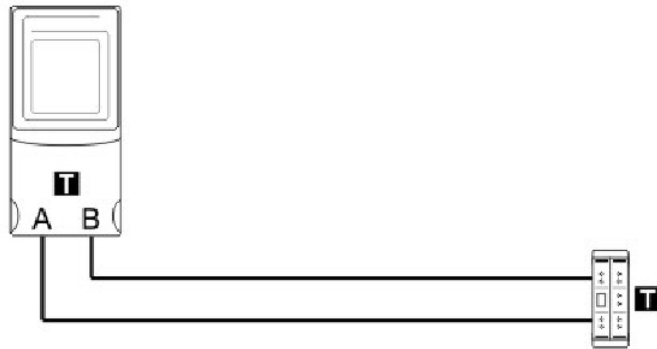
Figure 2 - Dual Trunk Media Redundancy
