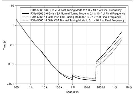
Tuning time refers to the time required to tune the preselector upwards in frequency. The time required to tune downwards in frequency can be 13 ms to 27 ms for RF center frequencies from 3.6 GHz to 7.5 GHz and can be 26 ms to 48 ms for RF center frequencies from 7.5 GHz to 14 GHz.
