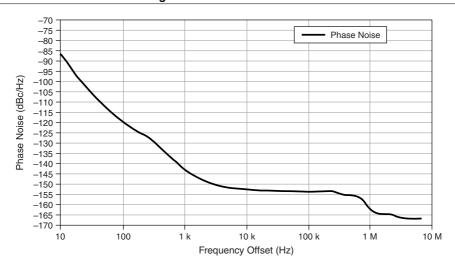
When used in a VSA system, the nominal specification for the VSA improves significantly from this value because the VSA uses all the LOs instead of a single LO. The phase noise of other LOs is correlated to the phase noise on LO1 at low offsets, which improves performance of the VSA system.
