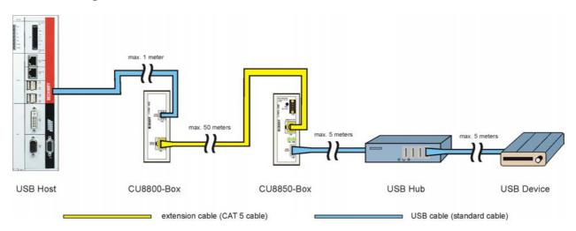
The USB hub is connected after the extension. The maximal distance is also 61 meters: 1 meter of cable from USB host to the USB extension box CU8800; up to 50 meters extension cable; 5 meters from extension box to USB hub and 5 meters of cable to the USB device.
