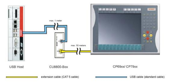
This configuration shows a CP69xx/ CP79xx Control Panel connected to the CU8800 extension box. The maximal distance of extension is 51 meters: 1 meter of cable from the host computer to the CU8800 extension box; up to 50 meters extension cable to the Control Panel.
