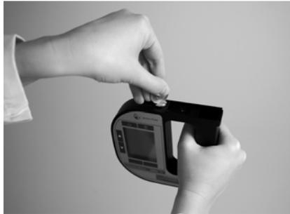
*Fig. 11 - 4 Opening the battery cover*
