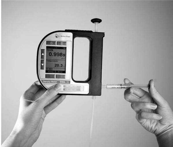
Fig. 9 - 2 Filling sample using the plastic syringe
