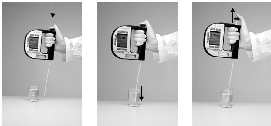
Fig. 9 - 1 Filling sample using the filling tube
