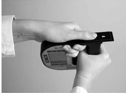
*Fig. 11 - 3 Removing the pump lock*
