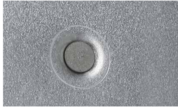
RESULT OF THE INSTALLATION OF SELF-PIERCING RIVET
