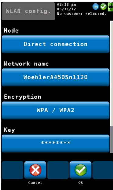
Fig. 35: WLAN configuration – Direct connection
