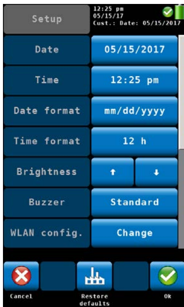
Fig. 33: Setup menu, the scroll bar shows that there are more parameters available.
