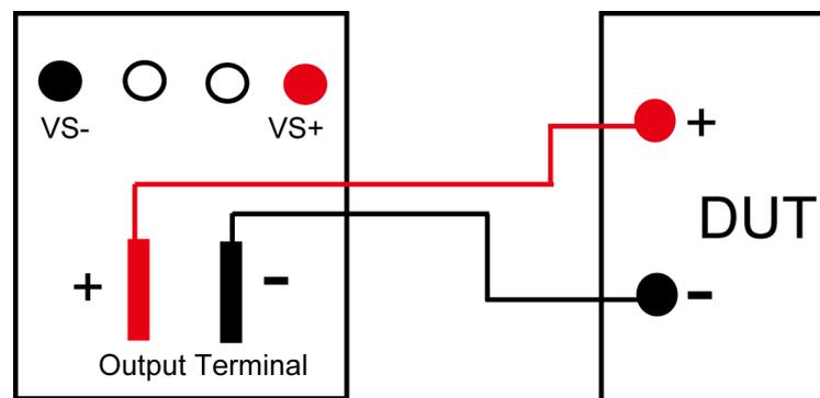
1. Confirm that the power switch is in the OFF position and verify that there is no dangerous voltage on the connection terminals.
