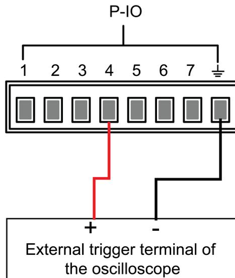
2. Set pin 4's function to **Not-Invert** and **Trig-Out**.
