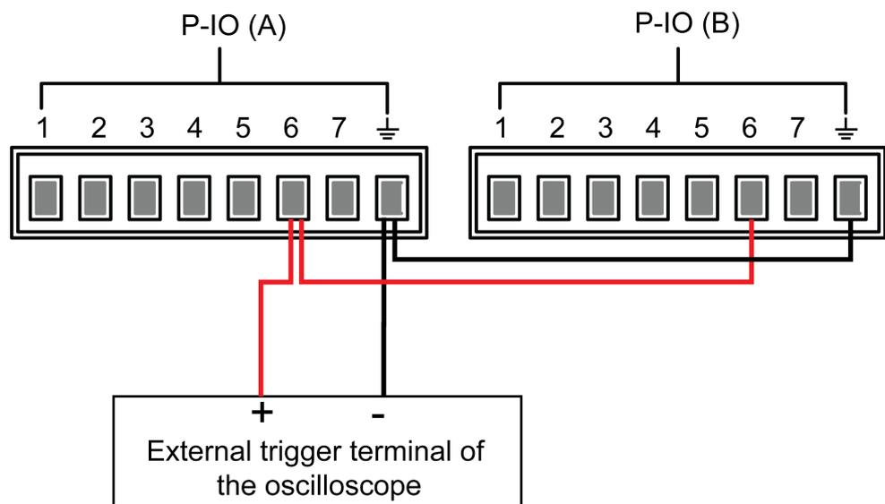
2. Set pin 6's function of two instruments to **Not-Invert** and **Sync-On**.
