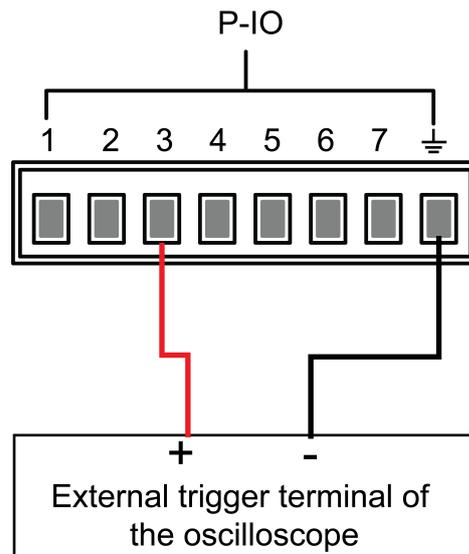
2. Confirm that pin 3 function is set to the default option, namely **IO-3. Off-Status, Not-Invert**.
