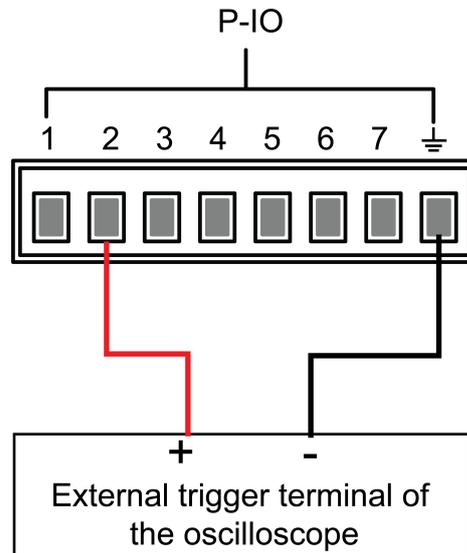
2. Confirm that pin 2 function is set to the default option, namely **IO-2. Ps, Not-Invert**.
