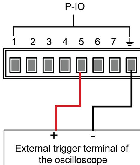
2. Set pin 5's function to **Not-Invert** and **Inhibit**→**Latch**.
