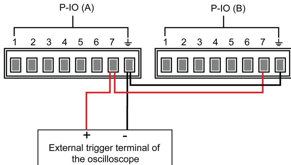
2. Set pin 7's function of two instruments to **Not-Invert** and **Sync-Off**.
