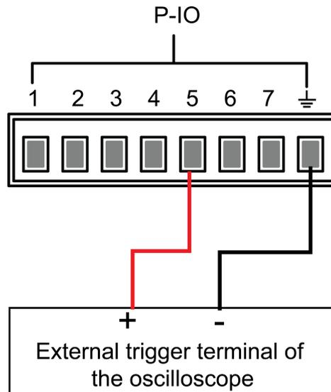
2. Set pin 5's function to **Not-Invert** and **Inhibit** → **Living**.
