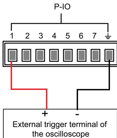
2. Confirm that pin 1 function is set to the default option, namely **IO-1. Ps-Clear, Not-Invert**.
