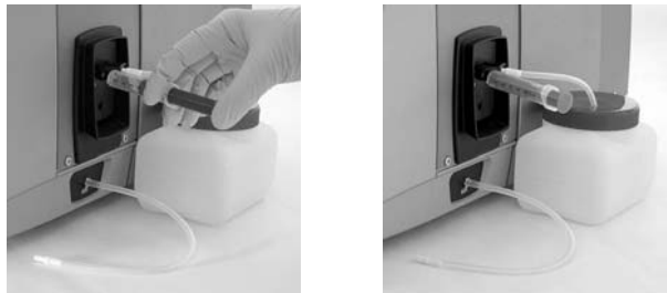
Fig. 10-2: Filling with a syringe
