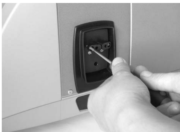
Fig. 7-1: Mounting the injection adapters Luer
