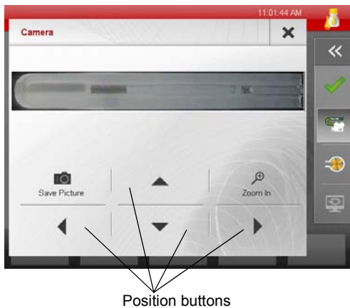
Fig. D - 1 Adjusting the camera position
