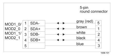
Figure 126 Dual RS-485 Module Wiring Diagram
