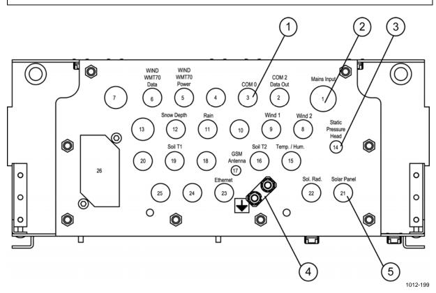
Figure 53 Connector Flange of the Enclosure
