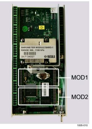
Figure 113 Communication Module Placement
