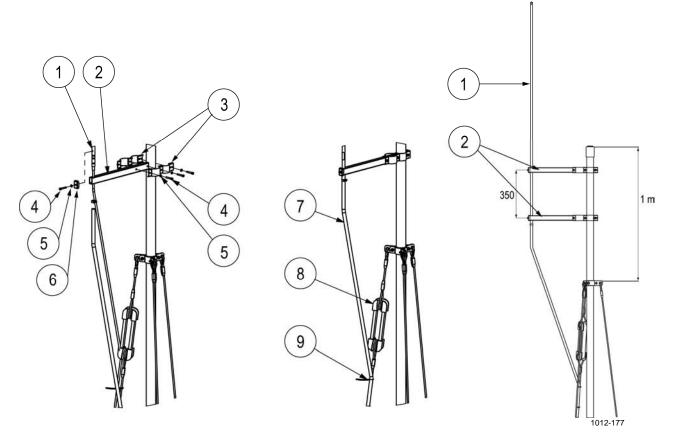
Figure 18 Lightning Rod Installation
