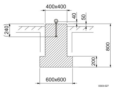
Concrete block dimensions for the guy wires are presented in Figure 7 below.
