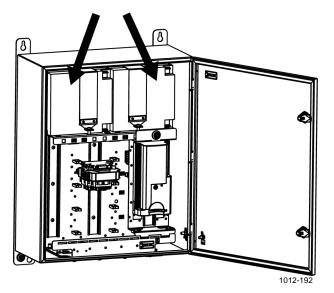
Figure 50 Backup Batteries Positioned Correctly
