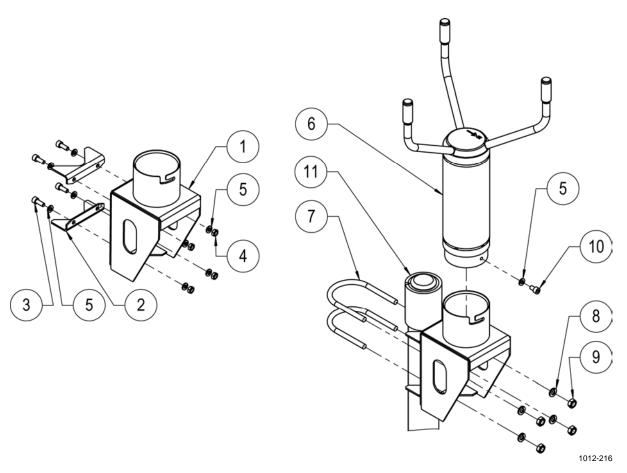
Figure 27 Installing Ultrasonic Wind Sensor WMT703
