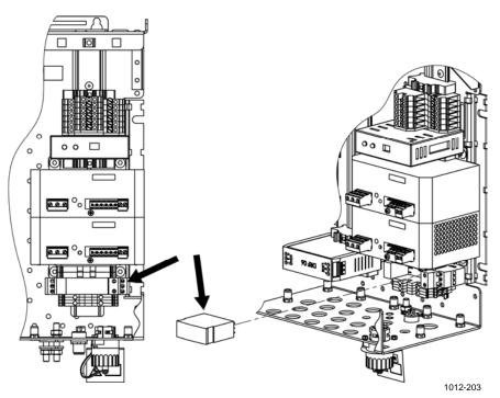
Figure 115 Removing AC (Mains) Power Surge Protector, Arrow Points to Surge Protector
