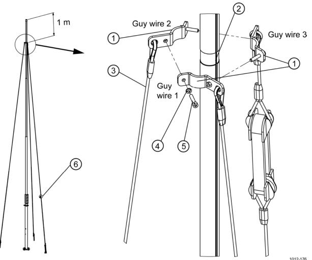
Figure 17Connecting Guy Wires to the Mast
