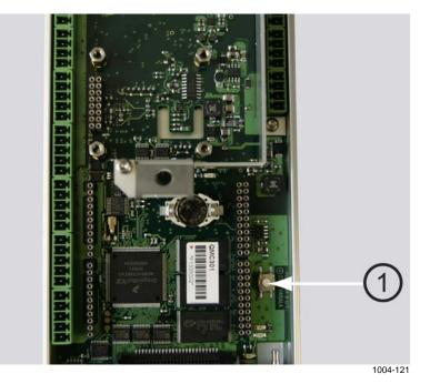
Figure 121 Reset Button on QML Logger
