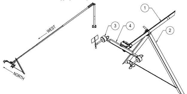
Figure 31 Installing Wind Sensors
