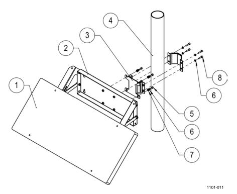
Figure 34 Installing Solar Panel SOLAR33
