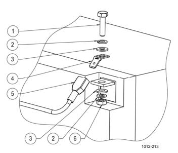
Figure 55 Connecting Battery
