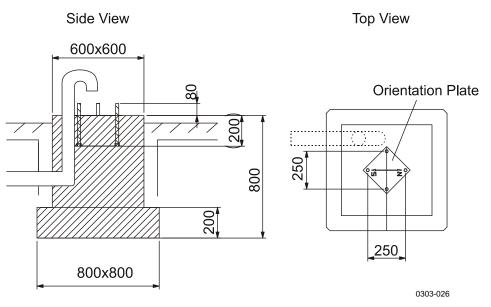
Figure 6 Main Mast Block and Orientation Plate (Dimensions in mm)
