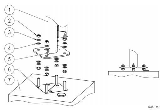
Figure 13 Pedestal Tube Attachment
