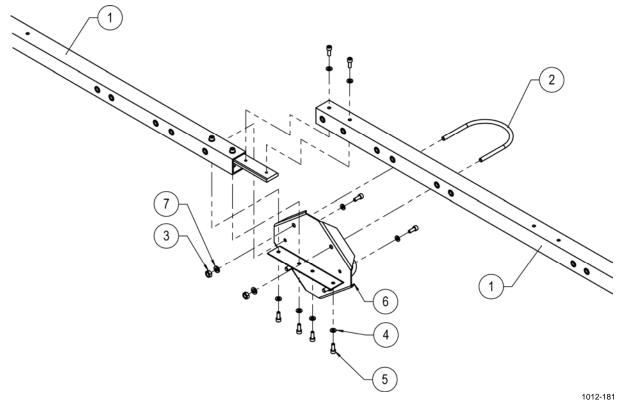
Figure 37 Mounting Sensor Support
