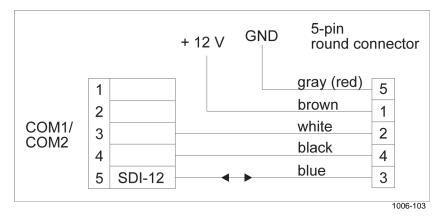
Figure 129 Dual RS-485 Wiring Diagram for SDI-12 and 12 VDC Power Supply
