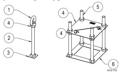
Figure 10 Foundation Assemblies for a New Concrete Block
