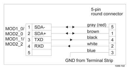
Figure 128 Dual RS-485 Wiring Diagram for RS-485 and RS-232
