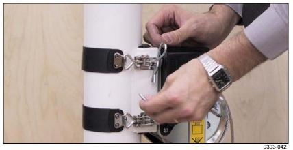
Figure 21 Securing Clamp of the Winch
