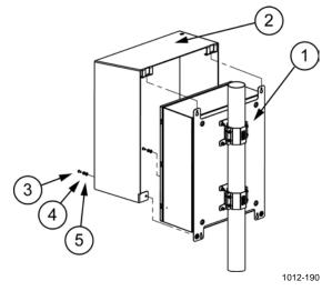
Figure 47 Installing Radiation Shield to Enclosure
