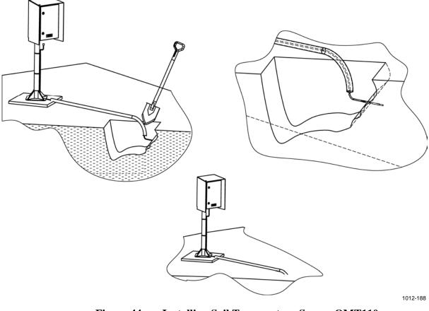
Figure 44 Installing Soil Temperature Sensor QMT110
