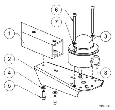
Figure 41 Installing Pyranometer CMP6
