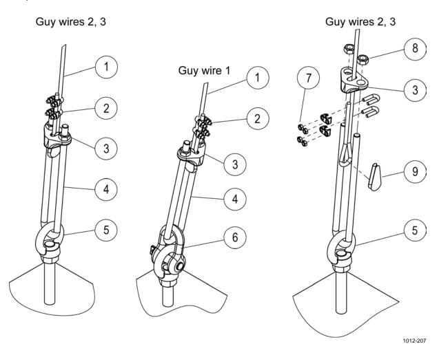
Figure 24 Connecting Guy Wires to Concrete Blocks
