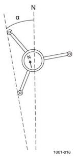
Figure 30 Incorrectly Aligned WMT703 and the Resulting Offset Error
