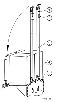
Figure 51 Attaching Strips over Battery
