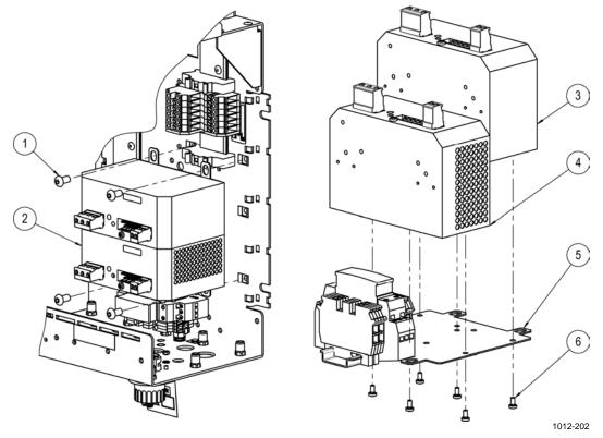
Figure 114 Removing Power Supply Set
