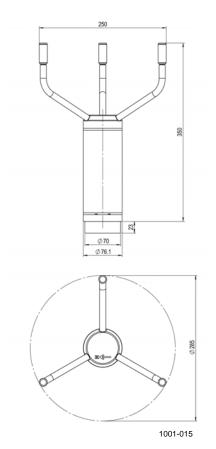
Figure 134 Ultrasonic Wind Sensor WMT703 Dimensions in Millimeters
