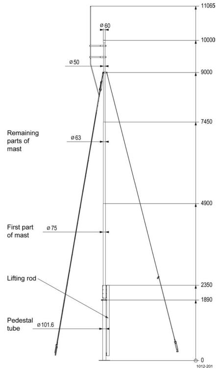
Figure 12 DKP210 Mast Dimensions (in mm)
