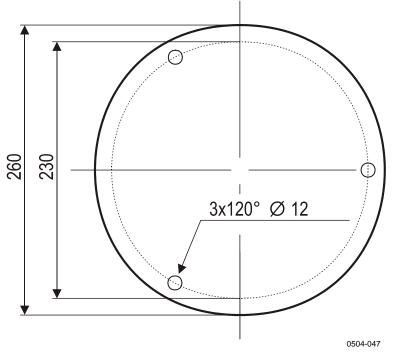
Figure 45 Installation Hole Placement for Rain Gauge Stand
