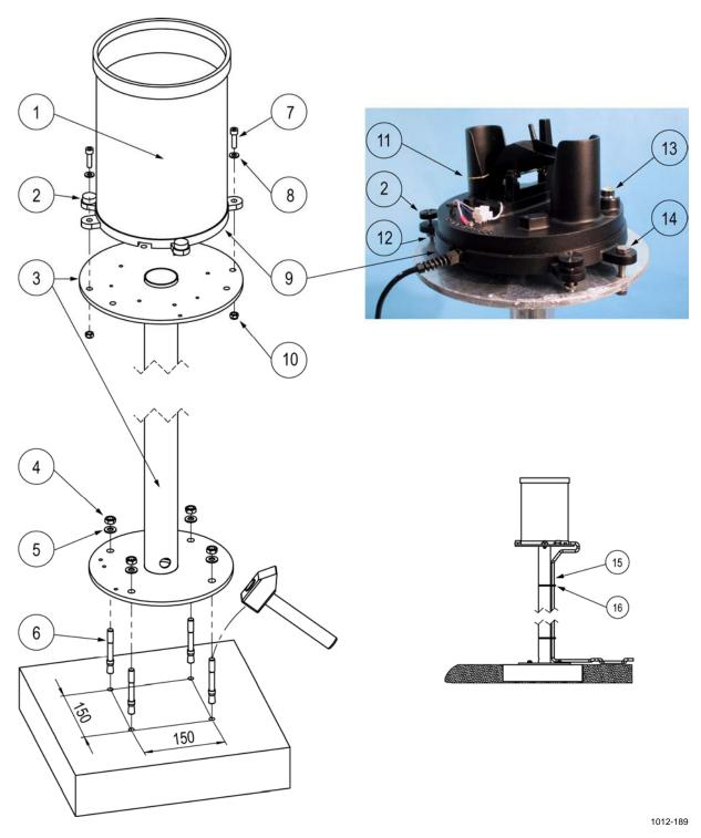
Figure 46 Installing Rain Gauge RG13(H)
