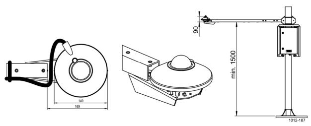
Figure 42 Pyranometer CMP6 Dimensions, Pyranometer CMP6 Installed
