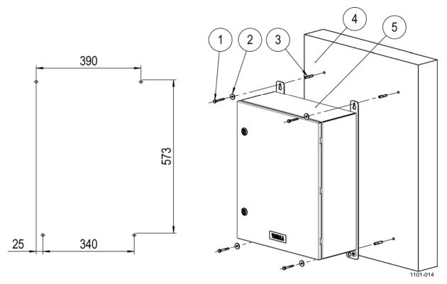
Figure 49 Installing Enclosure to Wall
