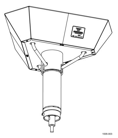
Figure 107 Testing WMT703 with Verifier
