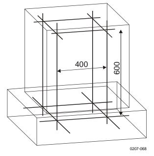
Figure 8 Reinforcement for the Concrete Blocks
