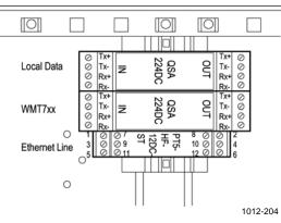
Figure 116 Removing Data Line and Ethernet Surge Protectors
