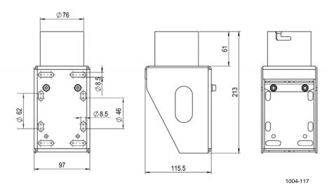
Figure 135 Mounting Kit FIX70 Dimensions in Millimeters
