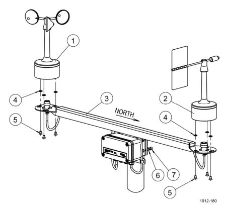
Figure 32 Mechanical Wind Sensor Set WA15 Installation
