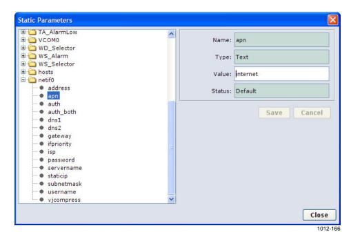
Figure 79 Setting GPRS Connection Parameters
