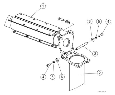
Figure 14Hinge Axle Installation
