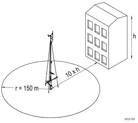
Figure 3 Recommended Mast Location in Open Area
