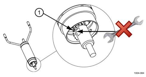
Figure 28 Tightening the Connector
