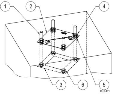
Figure 9 Foundation Assembly for the Mast Base
