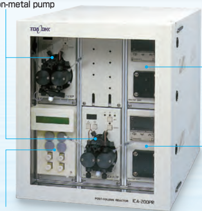
Inline degassing section
