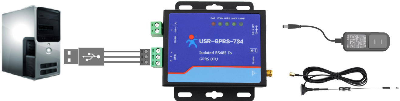
Figure 3 Hardware connection diagram
