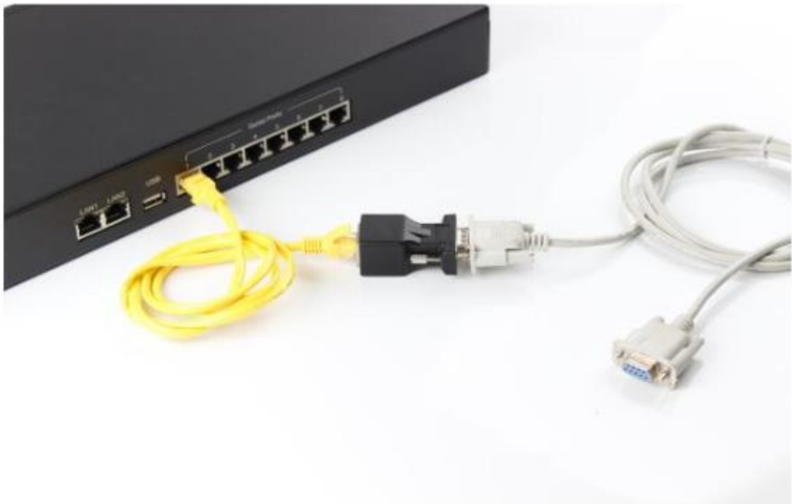
Figure 2. serial port connection between N668 and PC
