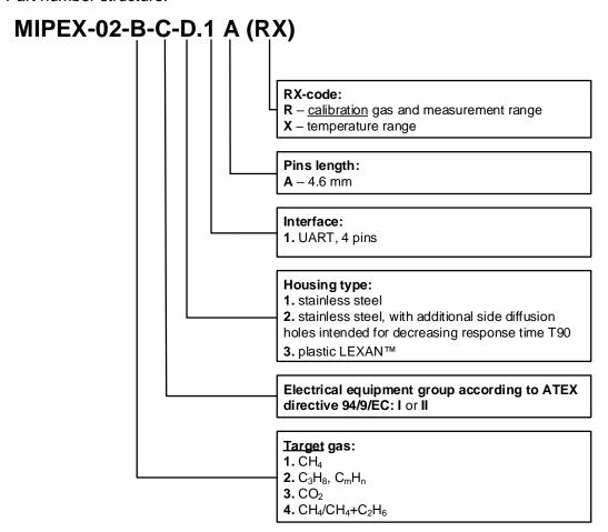
Term **target gas** refers to LED and photodiode spectral range, which is adjusted for best detection of a certain gas, while term **calibration gas** refers to gas mixture used for sensor calibration.
