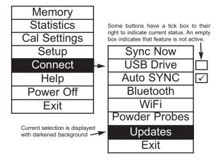
To navigate, use the Up and Down buttons to scroll vertically and [w] to SELECT.
