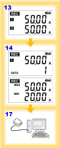
13 Hold REC/STOP on the logger for two seconds to start recording.
