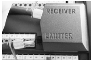
Fig. 4: SMA-connection to M800 transmitter "Receiver/Emitter".
