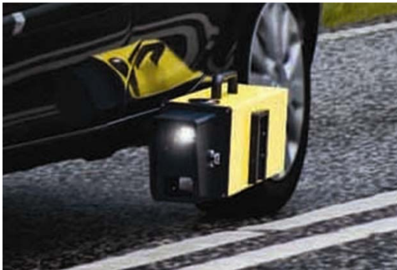
The LTL-M sensor mounted on a vehicle
