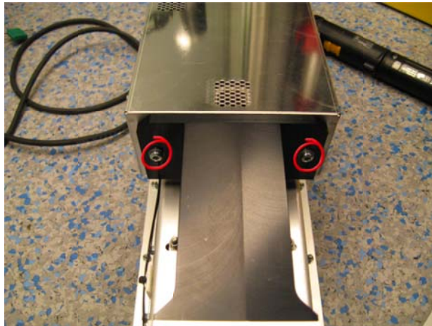
To remove the flash unit, unscrew the three marked screws.
