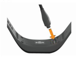
**3** Plug the USB cable into a power source to turn on the device (*Charging the Device*, page 8).
