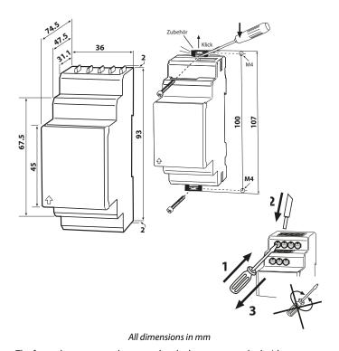
The front plate cover can be opened at the lower part marked with an arrow.
